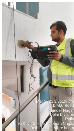
Photo 48: Half cell Potential Test is in Progress
