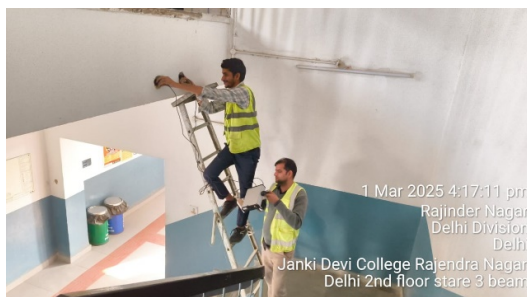
Photo 27: UPV Test is in Progress
