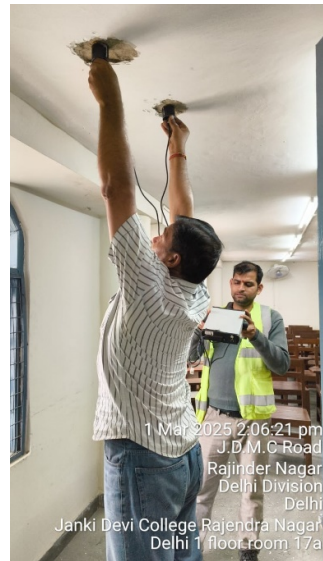
Photo 42: UPV Test is in Progress
