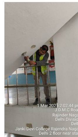
Photo 18: RH Test is in Progress
