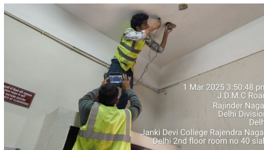
Photo 51: Half cell Potential Test is in Progress
