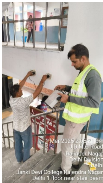
Photo 43: UPV Test is in Progress
