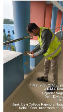
Photo 14: RH Test is in Progress
