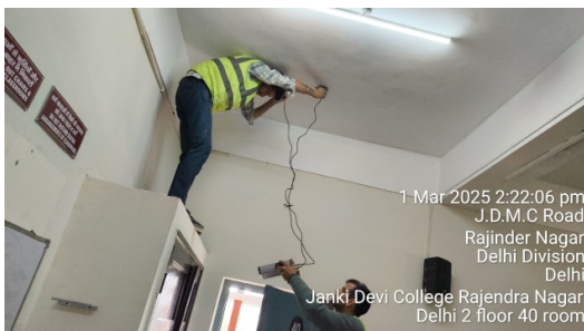
Photo 29: UPV Test is in Progress
