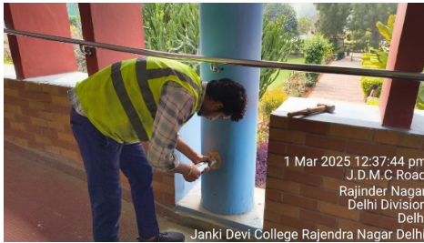
Photo 7: RH Test is in Progress
