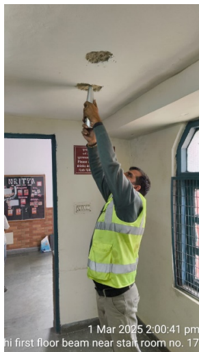
Photo 17: RH Test is in Progress
