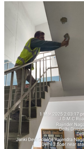
Photo 14: RH Test is in Progress
