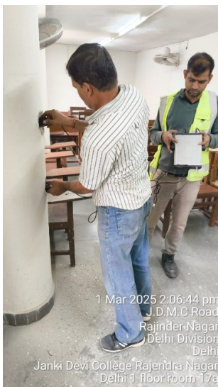
Photo 45: UPV Test is in Progress
