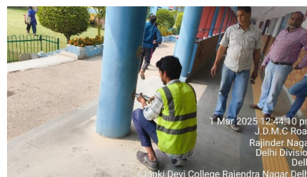
Photo 6: RH test is in Progress
