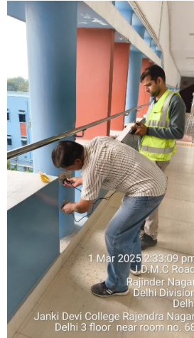
Photo 38: UPV Test is in Progress
