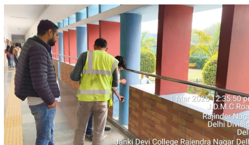
Photo 30: UPV Test is in Progress
