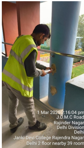
Photo 15: RH Test is in Progress
