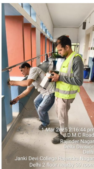
Photo 47: UPV Test is in Progress
