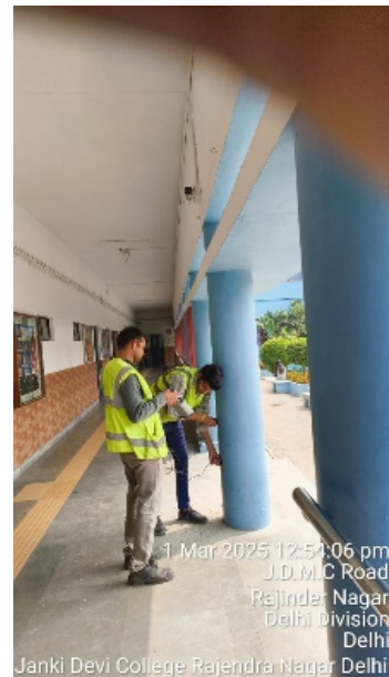
Photo 44: UPV Test is in Progress
