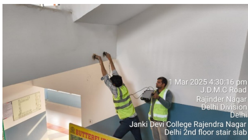
Photo 25: UPV Test is in Progress
