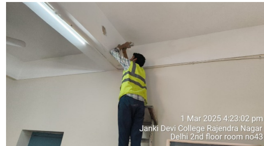
Photo 10: RH Test is in Progress
