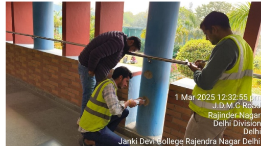
Photo 8: RH Test is in Progress
