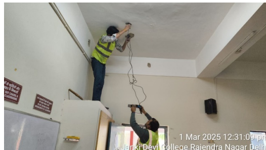
Photo 32: UPV Test is in Progress
