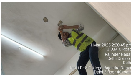
Photo 5: RH Test is in Progress
