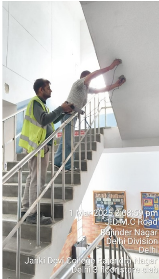
Photo 41: UPV Test is in Progress
