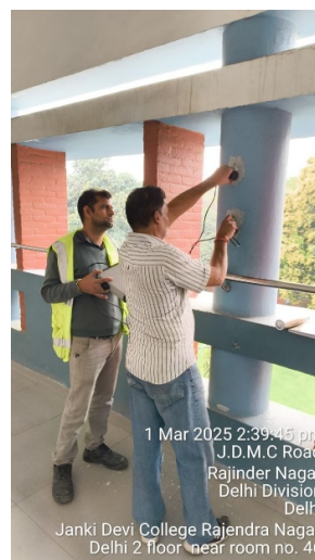
Photo 36: UPV Test is in Progress
