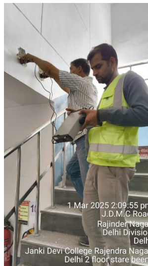
Photo 46: UPV Test is in Progress
