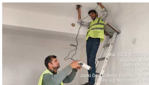
Photo 34: UPV Test is in Progress
