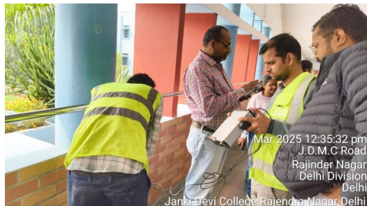
Photo 31: UPV Test is in Progress
