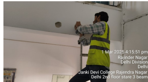
Photo 2: RH Test is in Progress
